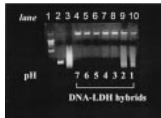
Figure 2. Electrophoresis analyses for the DNA-LDH hybrids with respect to pH. The pH of the solution dispersed with hybrid was adjusted to 7.5, 6.0, 5.0, 4.0, 3.0, 2.0, and 1.0, respectively, by adding 1 M HCl. After 1 h incubation of mixtures at room temperature, each sample was analyzed by 0.7% agarose gel electrophoresis and stained with ethidium bromide. Lane 1, \lambda -HindIII cut DNA marker (descent to 23.1, 9.4, 6.5, 4.3, 2.3, 2.0 kbp); lane 2, 500 bp DNA marker; lane 3, DNA; and lane 4–10, DNA-LDH hybrids at pH 7.5, 6, 5, 4, 3, 2, and 1, respectively.
